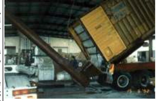
Figure 2 – Auger Unloading a Bulk Container
