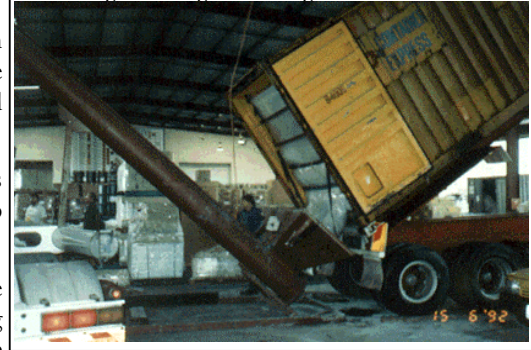
Figure 2 – Auger Unloading a Bulk Container
